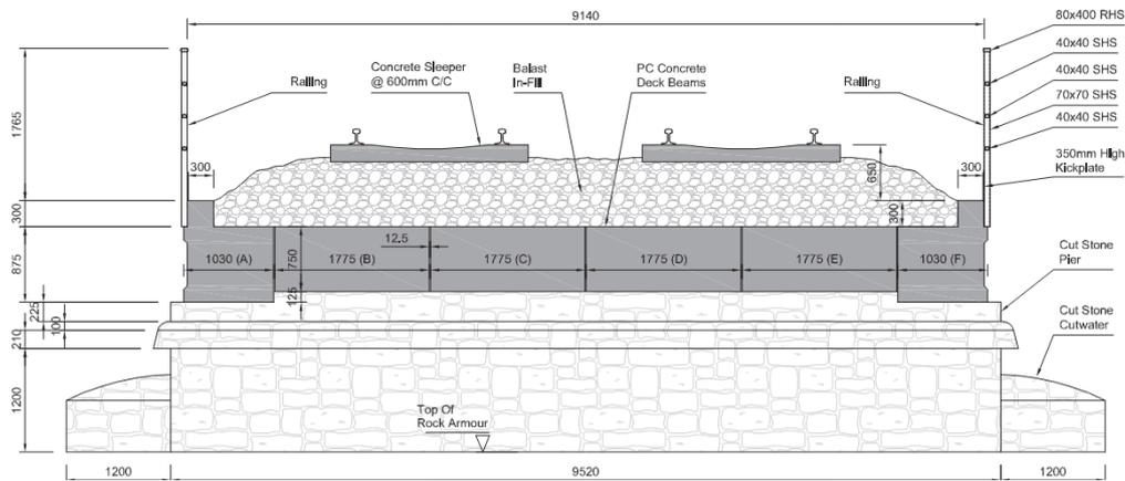
Figure 3-1: UBB30 Typical section for spans 1 and 12 (end spans)
