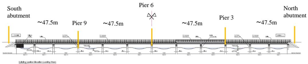
Figure 3-12: UBB 30 - Longitudinal frame arrangement 1 (preferred)
