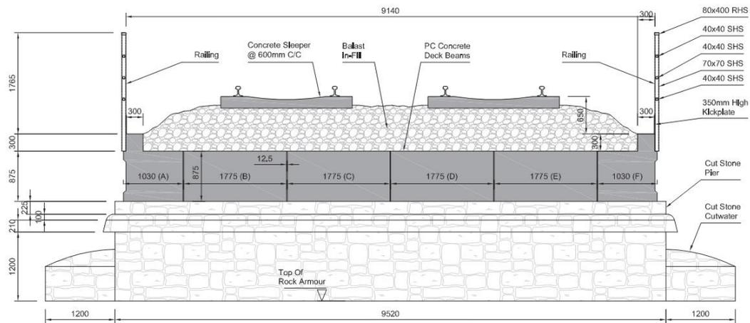
Figure 3-2: UBB30 Typical section for spans 2, 3 and 6 to 11
