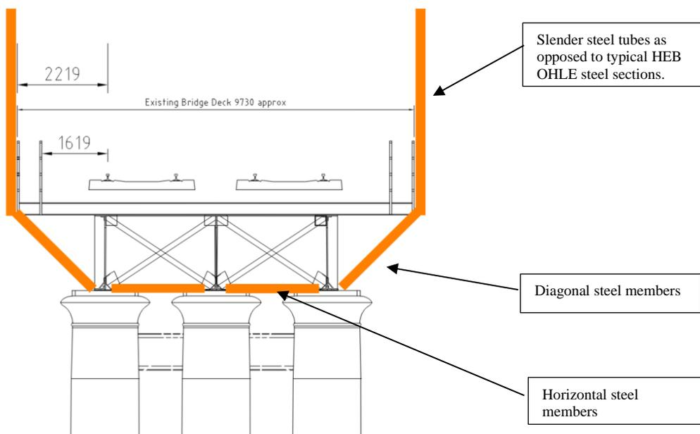
**Figure 7-14: Proposed OHLE option - cross-section**
