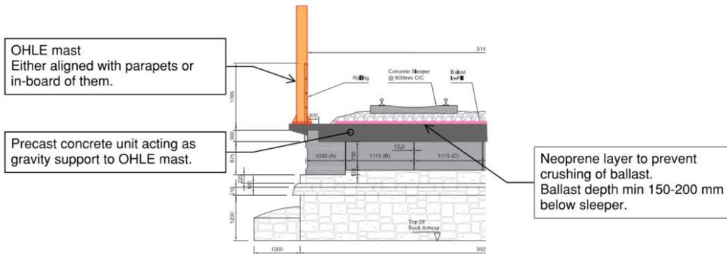
Figure 3-16: UBB30 – Proposed precast unit option (section)
