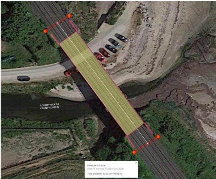
**Figure 6-7: UBB65 Aerial photo with deck (highlighted yellow and potential OHLE mast locations (red dots) at 60m spacing (Source: Google Earth)**
