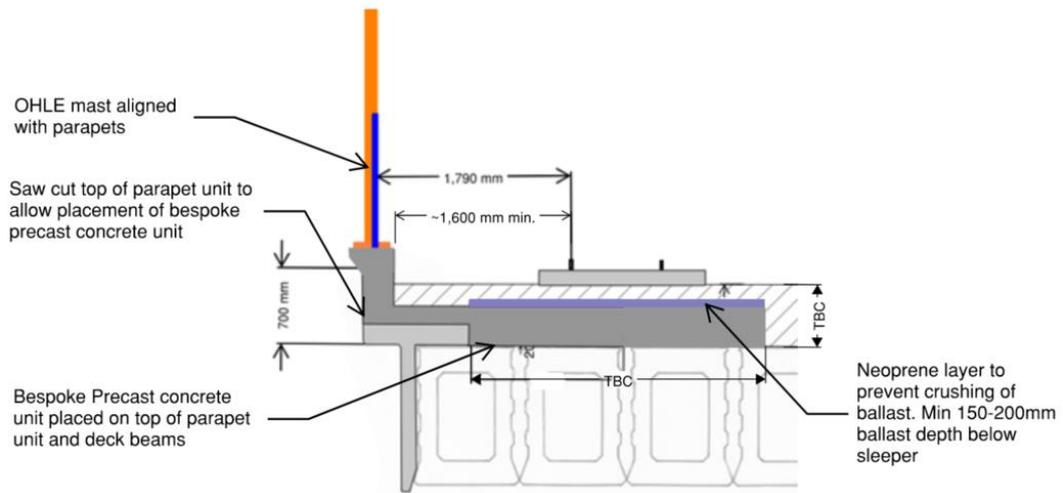
**Figure 4-11: UBB36 Proposed Option A**
