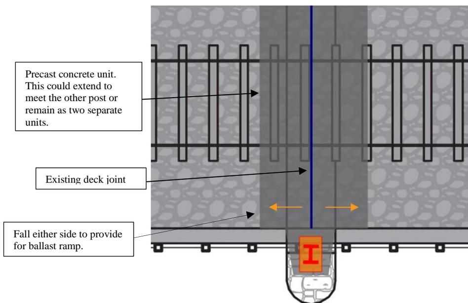
Figure 3-17: UBB30 – Proposed precast unit option (plan)
