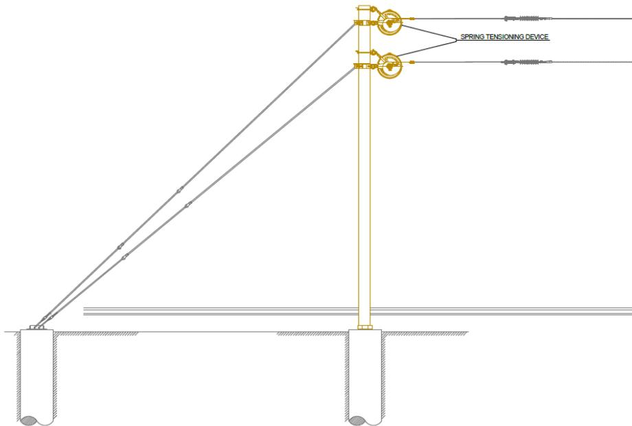
**Figure 2-3: Tensioning Device**
