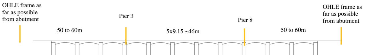
Figure 5-7: UBB56 proposed longitudinal framing arrangement
