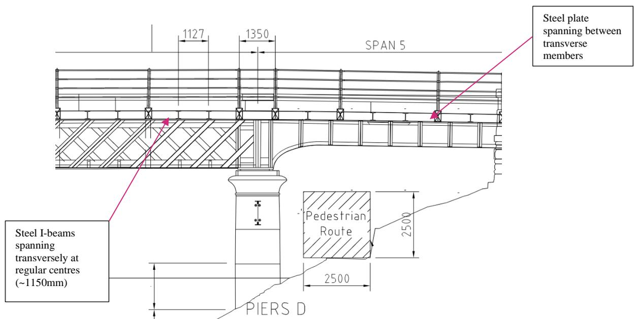
**Figure 7-1: UBB72 Side elevation drawing**
