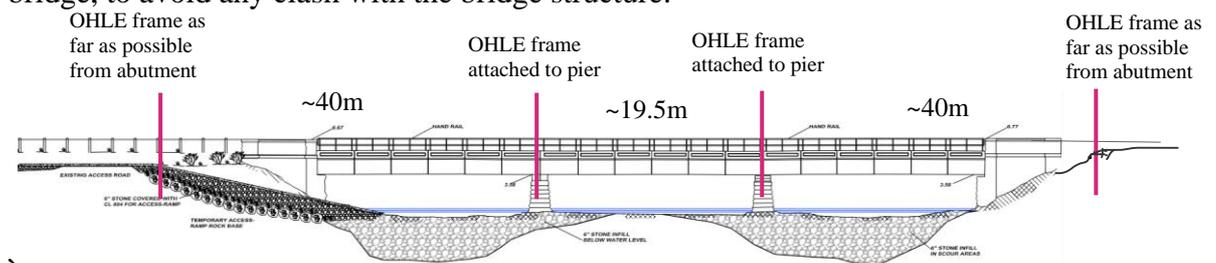
**Figure 4-10: UBB36 OHLE longitudinal arrangement – Arrangement 2**
