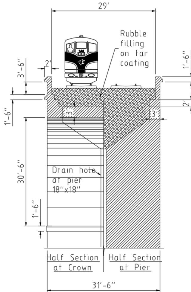
**Figure 8-2: Boyne Viaduct typical cross-section**
