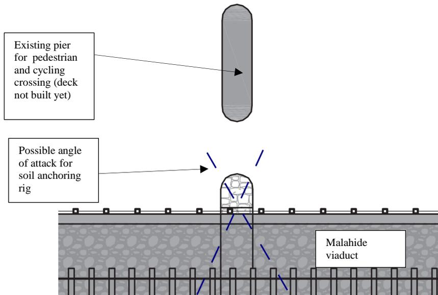
**Figure 3-21: UBB30 Ground anchors option (Plan)**
