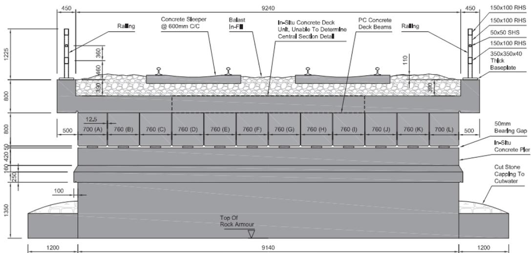
Figure 3-3: UBB30 Typical section for spans 4 and 5 (spans replaced following collapse)
