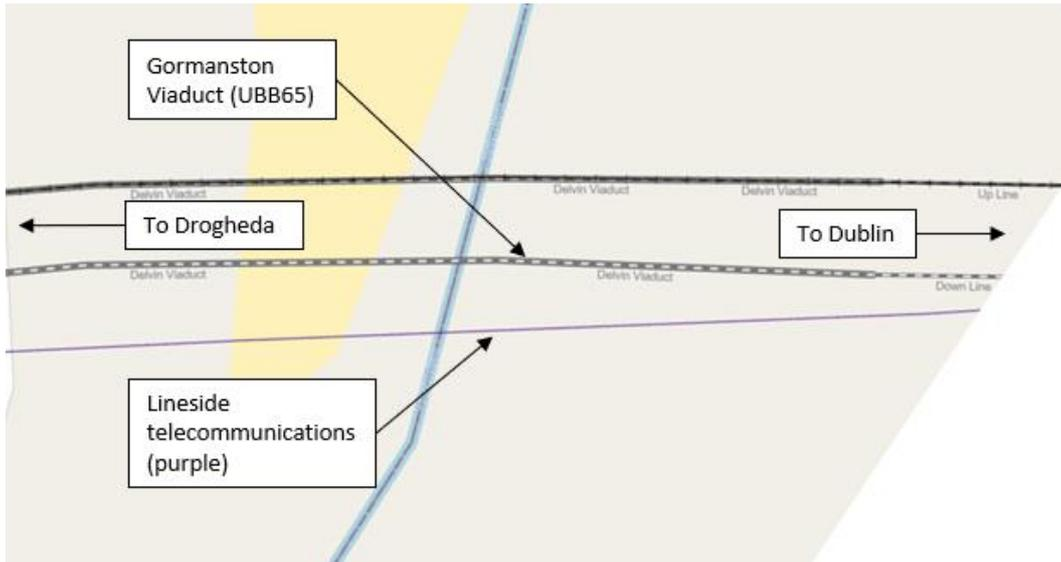
**Figure 6-5: Plan of Gormanston Viaduct (UBB65) showing existing utility routes (Map data © OpenStreetMap contributors, Map layer by Esri)**
