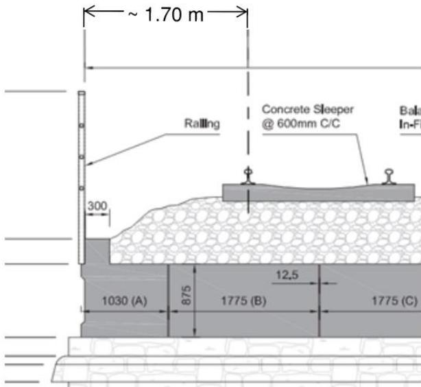
Figure 3-15: UBB30 Existing clearance to face of parapet
