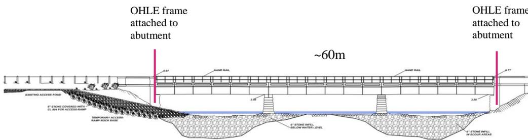
**Figure 4-9: UBB36 OHLE longitudinal arrangement - Arrangement 1**
