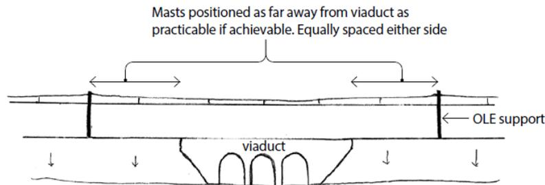
**Figure 2-1: Approach to longitudinal frame arrangement for underbridges with lengths < 60m**
