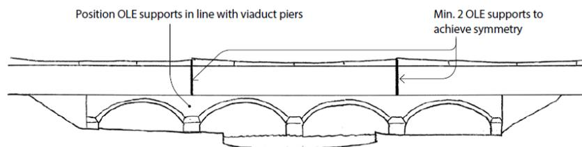
**Figure 2-2: Approach to longitudinal frame arrangement for underbridges with lengths > 60m**
